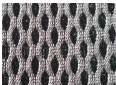
Figure 9 – Construction of spacer fabric
