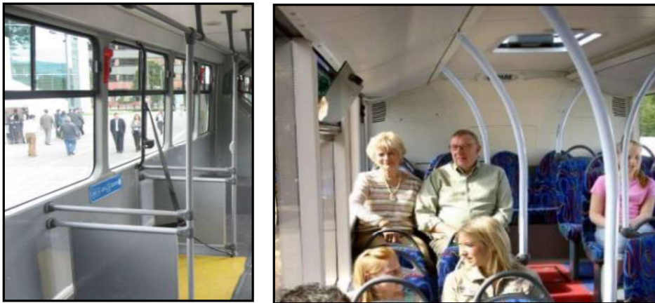
Figure 6: Examples of sliding vents (left) and hopper (right) vents.
