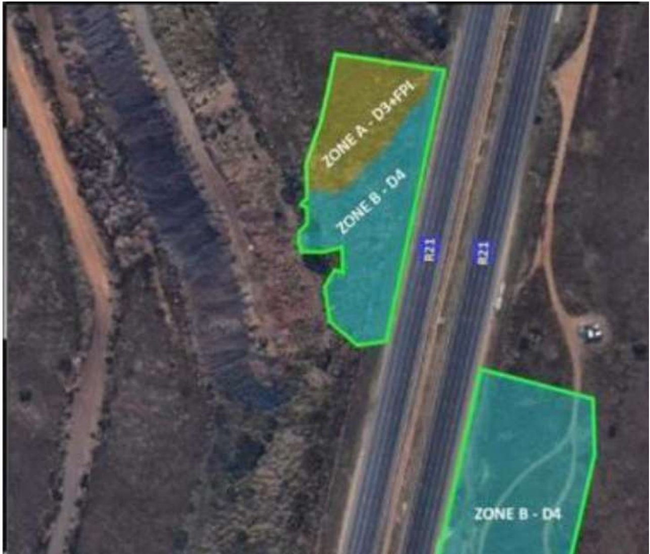
Figure 1-3. Apollo Croydon 1 275kV T17 R21: Dolomitic Designation
