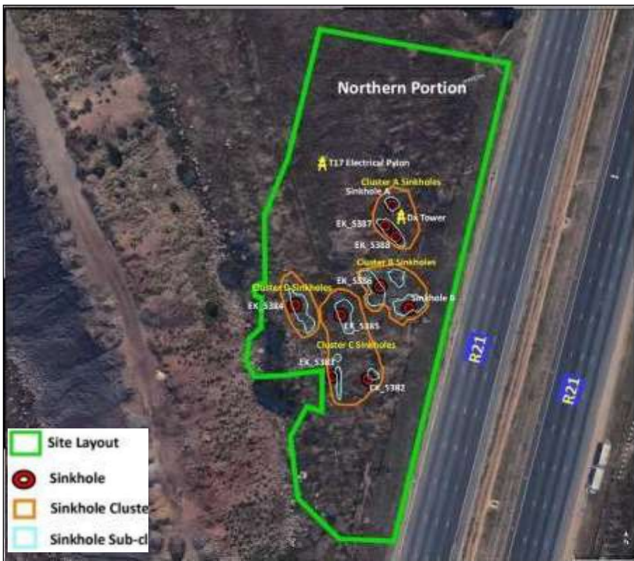
Figure 1-2. Apollo Croydon 1 275kV T17 R21: Area Layout depicting Clusters
