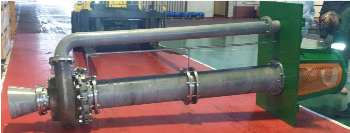
Fig.1: Tutuka P/S – Vertical Anion Supply Pump (3.0m length)
