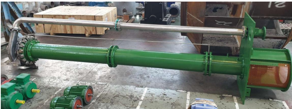
Fig.2: Tutuka P/S – Vertical Sandfilter Supply Pump (4.8m length)
