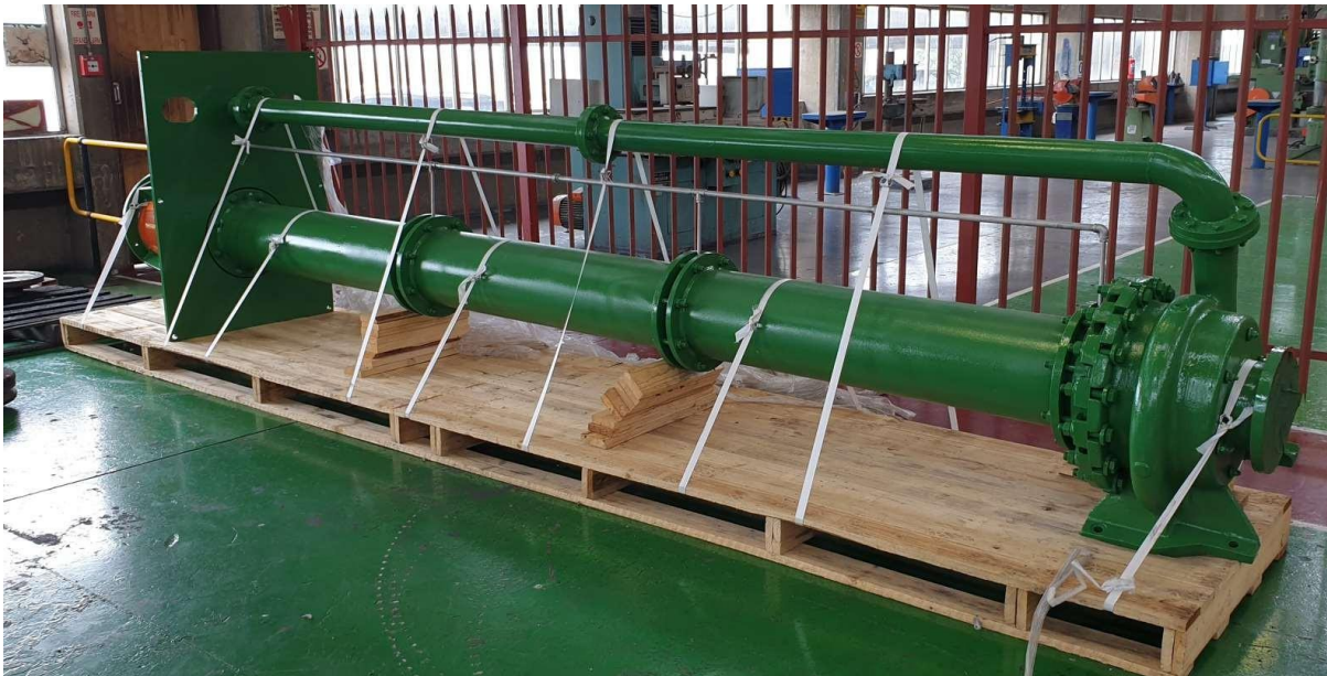
Fig. 3: Example of acceptable Packing and Crating during pump transportation/delivery
